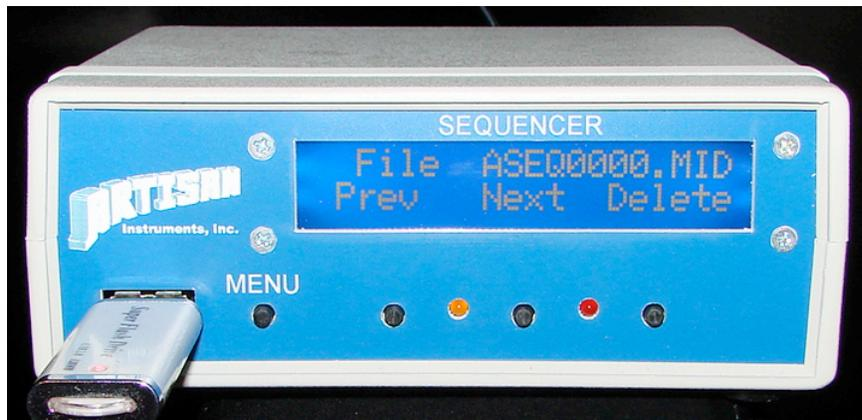
11. The DELETE button is also found on the Navigation screen. To Delete a MIDI file, first find it with the Previous and Next buttons and then press the Delete button. The screen will change to Delete – No – No. Press Delete to permanently delete the file. Pressing either of the No buttons will abort the deletion of the file and return you to the Main Record/Playback screen.
