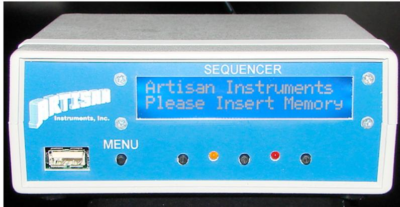
When you insert a memory, the menu screen will change to the Main Record/Playback screen. If any MIDI files are found on the memory, the name of the first file will be displayed on the top line.
