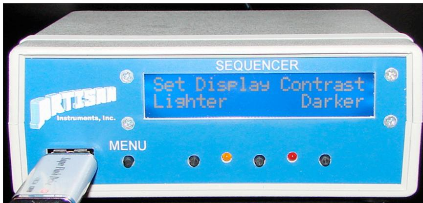
Pressing the MENU button again will bring you to the MIDI THRU screen. The top line of the display will report the current state of the MIDI THRU function. You may press the Enable or Disable button to change the MIDI THRU state.
