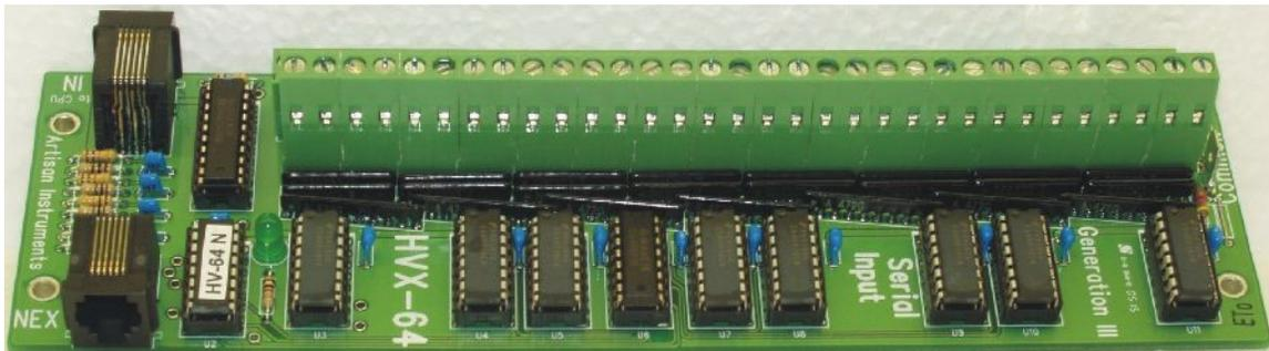
A microprocessor is added to give the board greater flexibility. The first major difference is that the inputs accept voltage levels, making it more suitable for organs that already have a voltage applied to their switch contacts. The HV-64P accepts voltages from 0V to 40V, and the HV-64N accepts voltages from -35V to +5V. The HV-64P can be used with switch closures to a common bus of +5V through 40V. The HV-64N can be used with switch closures to a common bus of 0v to -35V.
