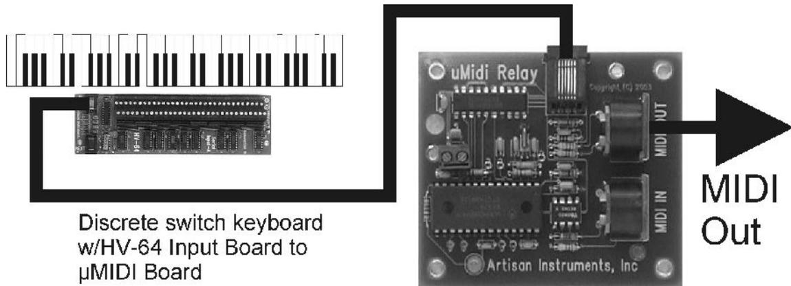
Up to 256 bits of input may be connected to one Micro-Midi interface board.
