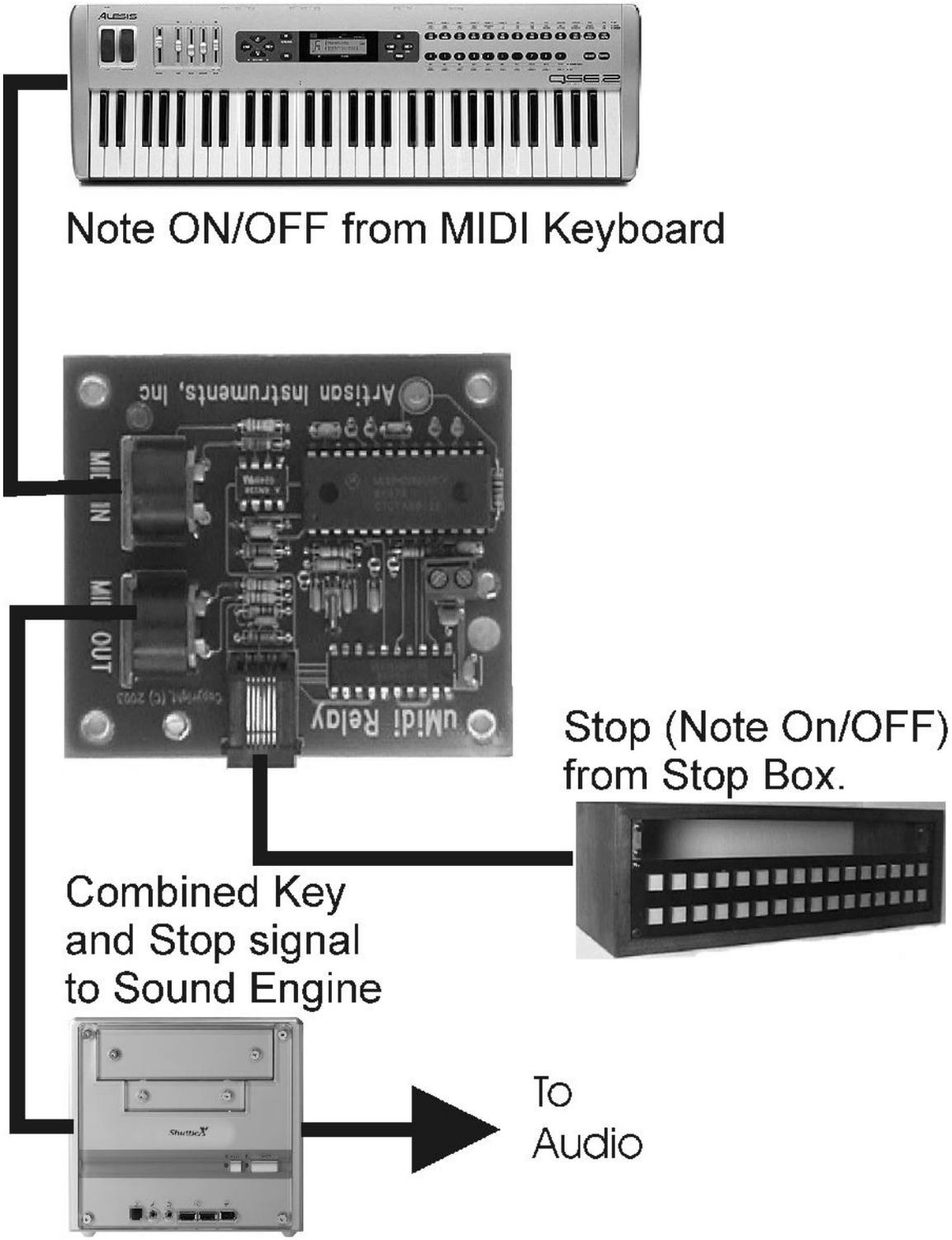
NOTE: If the MIDI information is originating from an organ that also sends out Note ON/OFF messages from its stops, then the Micro-MIDI Board is not needed for merging purposes.
