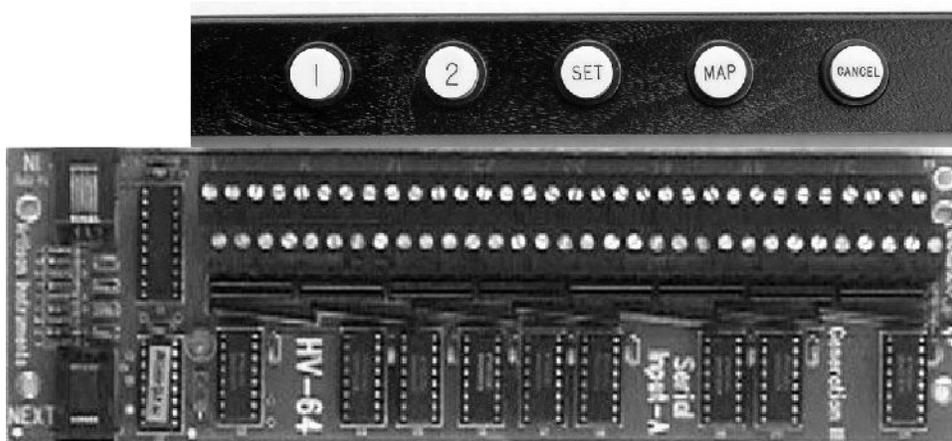
Thumb Pistons to HV-64 Input Board
