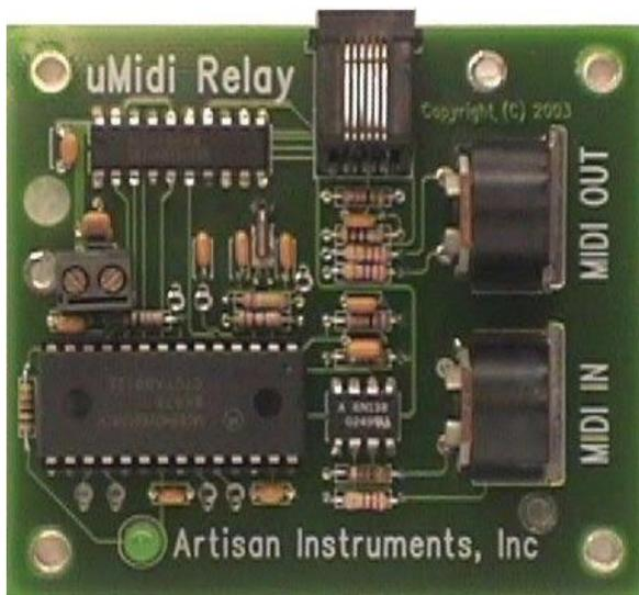
It consists of a board with (2) DIN connectors for MIDI IN and MIDI OUT, plus an RJ-11 connector for interfacing to other Artisan hardware.
