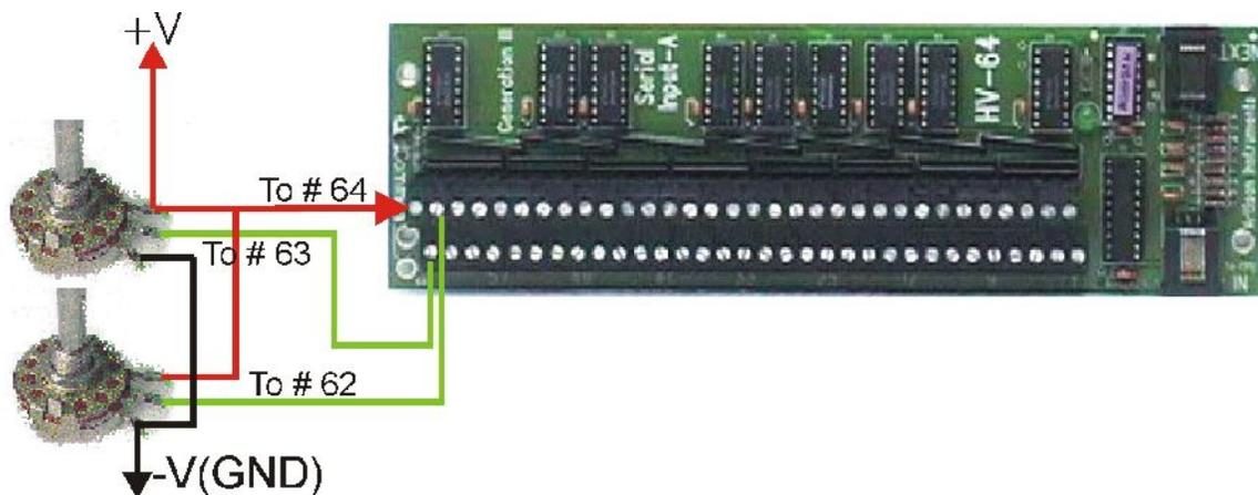
The second way in which a potentiometer can be added to provide volume, or expression, control is to connect the potentiometer wiper to the A to D input of the microprocessor on the Micro-MIDI Board. Up to four potentiometers can be connected to one Micro-MIDI board. (Earlier Micro-MIDI boards did not allow the connection of potentiometers.)
