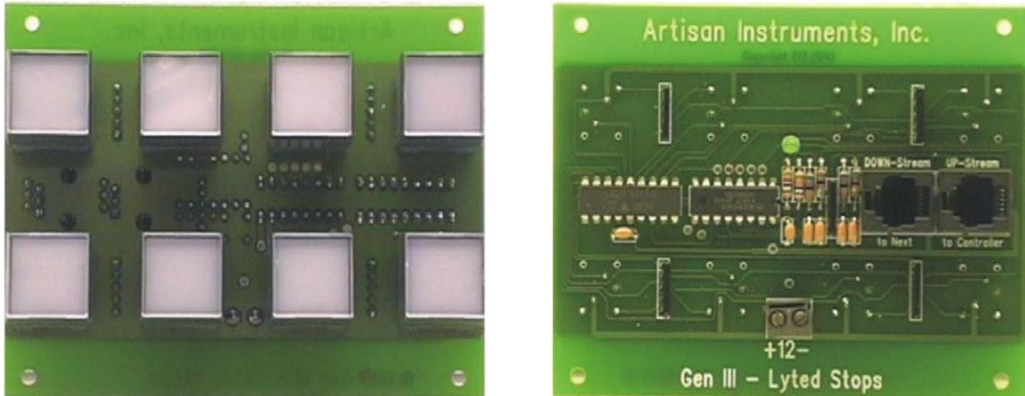
Further, as many as 8 Lighted Stop Modules may be connected in series to form a panel of lighted stop actions. The series group may be connected to a single Micro-Midi interface board.
