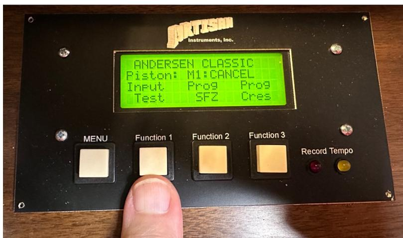
The Program Crescendo and Program Sforzando buttons will allow you to set stops on the different levels of Crescendo or SFZ piston. These buttons will only work if you have a working Crescendo Pedal and/or SFZ piston.
