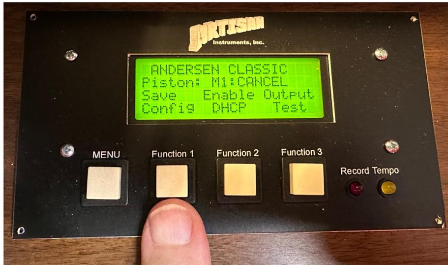
Save Config (Function 1) will save the operating file to your memory stick without having to connect via an Ethernet Cable.
