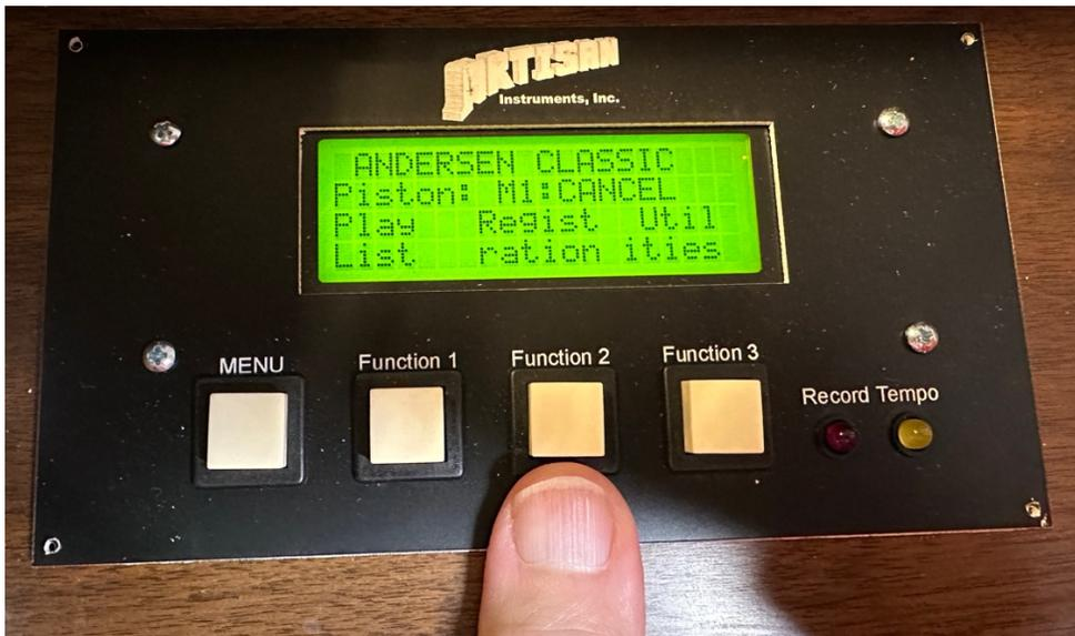
The Registration button allows you to save all your pistons to the Memory stick for later recall. When you press Registration (Function 2) a screen will pop up to allow you to save or load a registration that has been previously saved.
