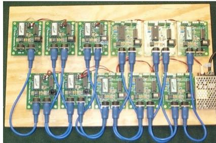
The second type is a 6-wire, flat phone cable used to connect Input Boards to a  $\mu$ MIDI Controller, or from a  $\mu$ MIDI Controller to a Driver Board. These cables can vary in length, depending upon the location of the Input Boards or Driver Boards with respect to their associated  $\mu$ MIDI Board.
