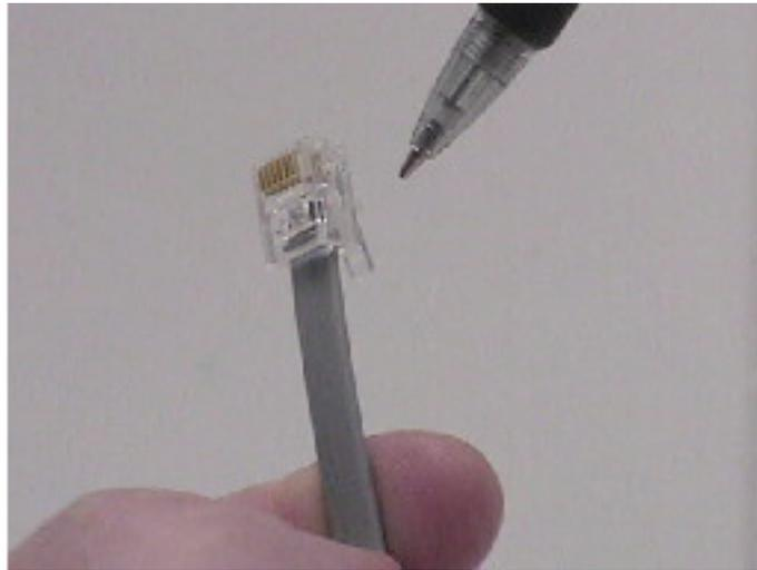
4) Crimp the connector tightly with the crimping tool. This method provides the proper orientation for the cables when plugged into the receptacles on the Micro-MIDI board(s) and the various other boards. In effect, it provides the 180 degree twist in the cable ---- which is correct.
